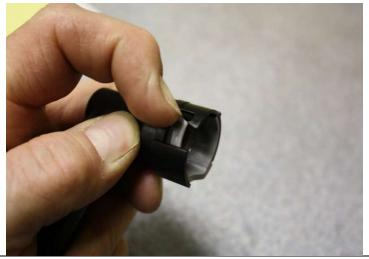
Locate tab below, this is on the passenger side of the radiator support. Push threaded J clip over hole, it will snap into place. The threaded portion should be on the underside of this tab. Install bracket and bolt into threaded portion. Slightly rotate bracket towards driver side of vehicle. Pay close attention that the bracket isn't sitting against the small coolant hose.
