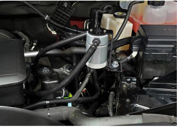
To properly clean the filter in the Oil Separator, spray any degreaser or solvent through it and let it air dry. Clean it every 10,000 miles.
