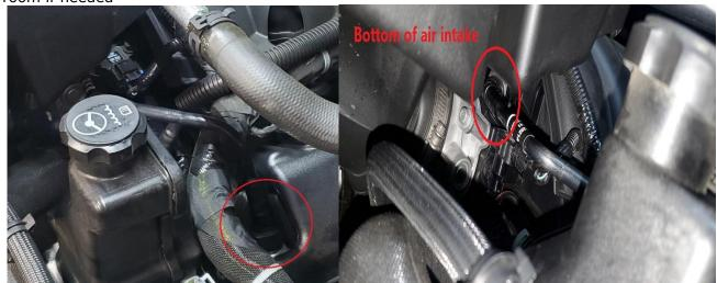
Mount J&L Bracket to auxiliary battery mounting bracket with the supplied bolt. **Note**: If your truck is optioned with the auxiliary battery, remove bolt securing this bracket and use the same bolt to mount the J&L Oil separator bracket.
