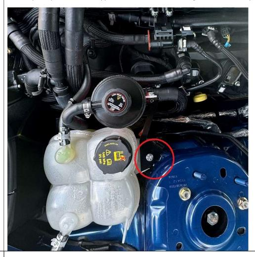
Pull EVAP solenoid off its bracket. Route long hose to intake pipe.
