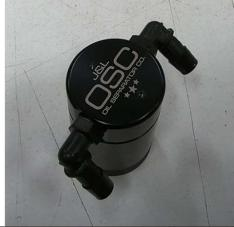
**3** Page 1 Lubricate both fittings on oil separator with light oil or grease, and lube inside of supplied hoses with the same. (Q-Tip works well for this).
