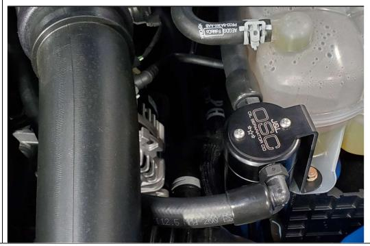
Route short hose with 90 degree quick connect to the intake connection and push to connect.
