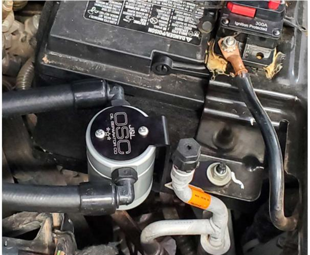
Route shorter hose to the intake connection and push to connect. The hose should route under the intercooler charge pipe and about the small coolant line. (See picture below)
