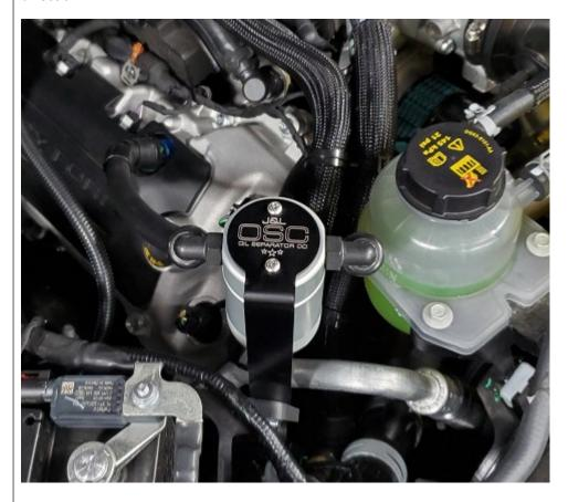
Route shorter hose to the valve cover connection and push to connect.
