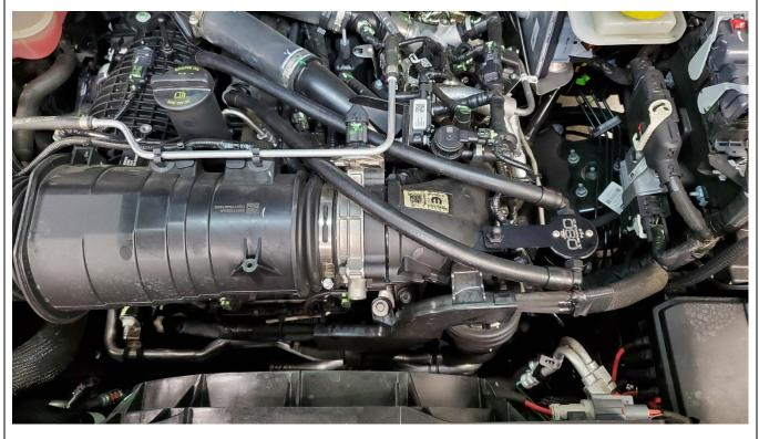
Reinstall the engine cover, check alignment of oil separator and snug down ball stud to secure the bracket/oil separator assembly. Use care to not overtighten this bolt as it's going into plastic, it needs to be tight enough to ensure the oil separator isn't sliding back and forth loose!
