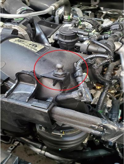
Feed oil separator hoses through the top of the engine, both hoses will run under the metal coolant pipe, the hose closest to the rear of the engine will feed between a wiring harness and plug as seen in the photo below. Install oil separator assembly into place and secure with ball stud removed earlier, do not tighten completely yet.
