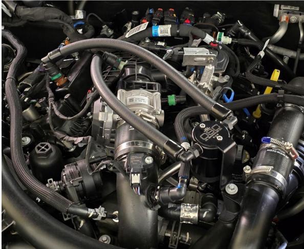
To properly clean the filter in the Oil Separator, spray any degreaser or solvent through it and let it air dry. Clean it every 10,000 miles.
