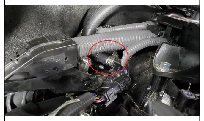
Reattached wiring harness to support.
