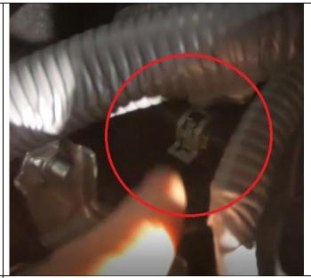
Use right angle needle nose pliers to slide factory clamp down PCV hose, once the clamp is slid down you may need to twist the hose to break the "seal". However, the hose may just pull right off.
